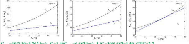
$G_{min}=10/2.10=4.762 \text{ kg/s}, G=1.4*G_{min}=6.667 \text{ kg/s}, L/G=10/6.667=1.50, CTC=2.7$
