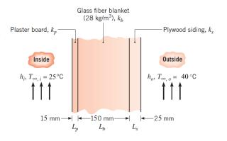
a) Calculate the heat transfer rate into the house
