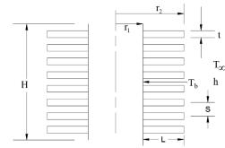
has a thermal conductivity of 60 W/m.K. Calculate the suface overall efficiency and the heat rate.
