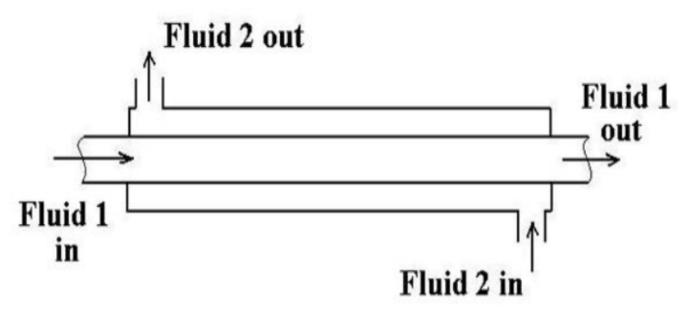
The objective is to design a double pipe heat exchanger i.e. finding the heat exchanger heat transfer area (which include the inner tube inside diameter, the heat exchanger length which fulfils the heat load and not exceeding the maximum pressure in the tube or annulus flow
